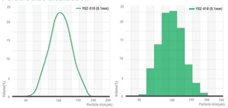
The result of measuring the particle size distribution shows a normal Gaussian distribution plot with left and right symmetry. Due to the narrow distribution, dispersion efficiency and quality are also improved.
